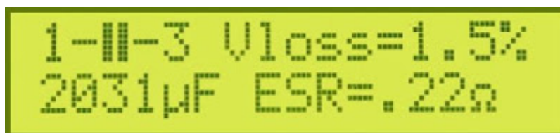
The measured parameters when testing an electrolytic capacitor with the MK-168.
